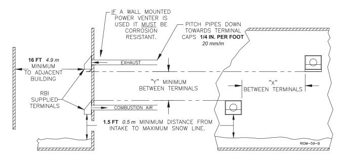
When running horizontal combustion air and venting for single or multiple units, exhaust and combustion air terminals must be installed on the same plane (outside wall) in order to prevent pressure differences due to prevailing winds. In cold climates, double-wall or insulated inlet pipe recommended to prevent condensation.
