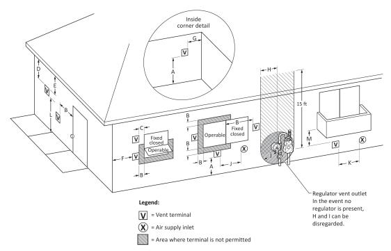
**Figure A - Direct Vent Terminal Clearances**
