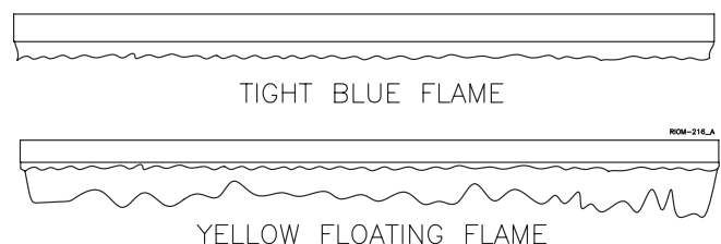
Figure 20 - Main Burner Flame
